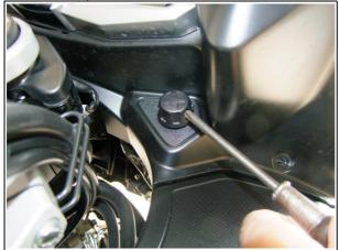
Carefully pop the centre panel loose along the top near the gauge cluster. Then slowly move outwards prize the centre panel in along the edge where it meets the fairing edge to pop the tabs loose. You'll need to open the glovebox lid to get it past the left side. Pull it up towards the cockpit for removal. With a little prodding it will come out.
