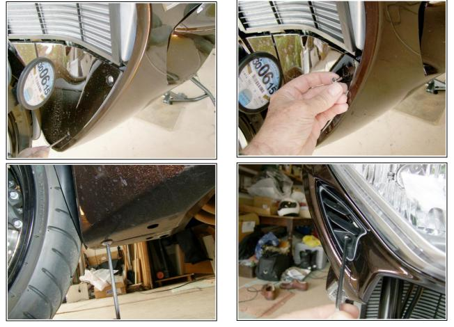
Remove the adjustable fairing venting on each side of the fairing – undo the quick-fasteners ...
