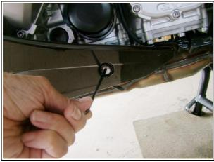
Remove the Philips screw from in front of the glovebox.
