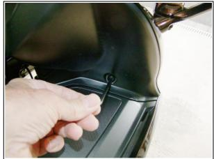
Remove the push pin fasteners that hold the centre dash plastic to the side panels on each side down along the fork tubes. While you are there remove all of the other push pin type fasteners you can see down there on the edges of the side panels.
