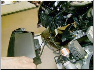
To reinstall, work backwards through the removal procedure. Take care with getting all tabs tucked in correctly. Easy to get wrong, e.g. where the two fairings join underneath.
