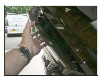
Remove the fasteners at the bottom trailing edge of each side of the fairing. Lying down helps to see them, one on each side.
