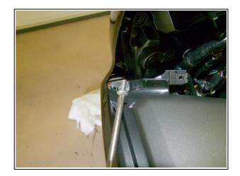
The last fastener to remove is the one hiding behind the adjustable side panel. Remove it. You are now ready to remove the left side fairing.
